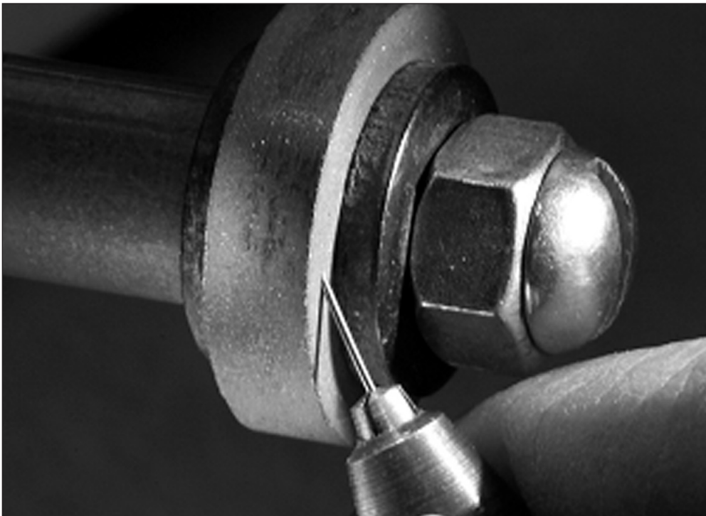
Figure 20. The needles are sharpened on this diamond impregnated rubber wheel that is mounted on a miniature Foreman bench grinder. The wheel rotates away from the acute edge and final touch-up is done on silicon carbide wet or dry sandpaper 1000 grit or higher.
