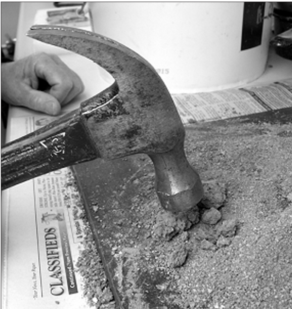
Figure 3. Matrix, processed to make aggregate for the system, was pounded with a hammer on a steel plate and the crushed rubble swept onto the newspaper underneath it.
