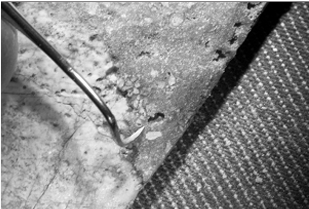
Figure 7. Everything must be done in a quick but fluid motion under the microscope. This is a dry run to visually locate everything so there will be no searching to bring the pick into the field of view during the real thing. The object, in this instance, is to fill the void seen at the sharp end of the pick. But the same method is used in filling cracks. The specimen rests on a sandbag made of denim.
