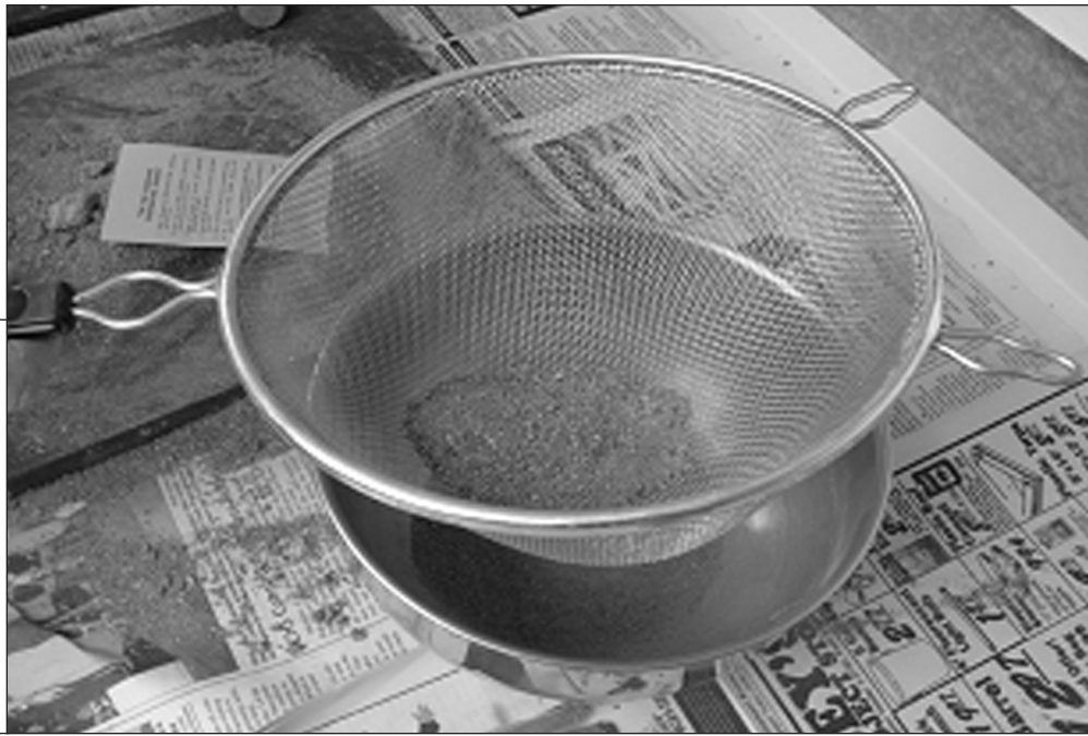
Figure 4. The rubble is then put through a 14-mesh (14 openings to the inch) kitchen strainer. This produces the large grain fraction of the aggregate we will use. It is what you see in the bowl under the strainer.
