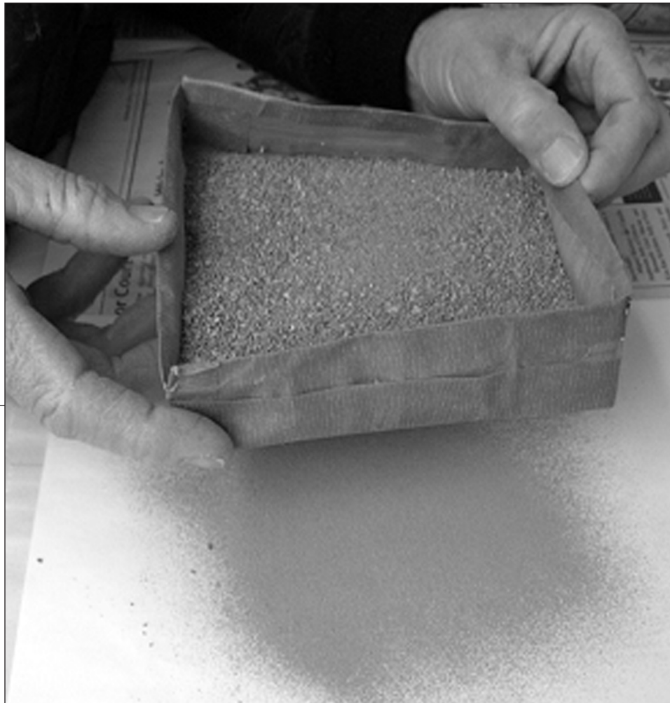
Figure 5. Some of the large grain fraction is then put through a 30-mesh strainer producing the fine grain fraction. What we are producing is something like the sand and gravel used as aggregate to mix with Portland cement and water to make concrete. They make it stronger. Another similarity here is that by using only the fine grain fraction a sort of superglue mortar is produced for filling and adhesion in very small gaps.
