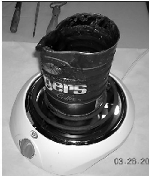
Figure 3. Coffee can used to heat wax. The rim has been bent to form a pour spout.
