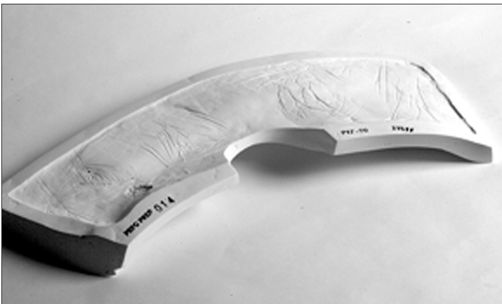
Figure 24. Plaster cradle to support the specimen in collections. The cut-out allows thumb and forefinger to grasp the piece for easy removal and replacement.
