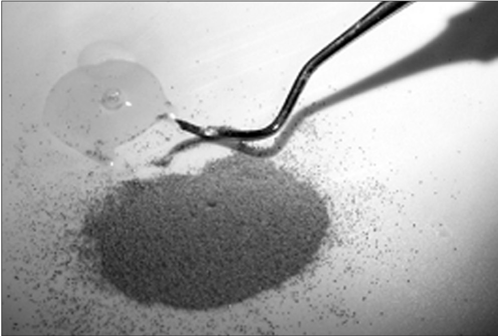
Figure 6. This is how the “mortar” is mixed on top of a dental mixing pad of treated paper. After each batch the top sheet is torn off exposing a new clean sheet. A large drop of cyanoacrylate (PaleoBond number 750) resin is placed next to a pile of the ground matrix that’s about 30 percent large grain and 70 percent small grain. This will allow two or three sub batches but the aggregate greatly accelerates the curing time. Once the two are mixed, there are only seconds available to place it. Some of the resin is mixed with the matrix and held as a drop in the bend of the dental pick. It will flow off when touched to the work.
