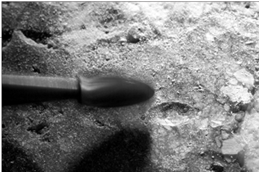
Figure 18. The excess filler must now be carved away. The blur in this picture is a spinning, 1/8 inch shank, single cut, oval head, carbide burr chucked in a pneumatic pencil grinder. This is used for roughing-out or bulk removal. If you always keep it moving in a circular pattern and start doing this in the air before touching down, you can produce a nice even surface like that in the right hand third of the image. But if you ever stop it will dig a divot like the one under the burr. This takes practice that should not be done on real specimens.
