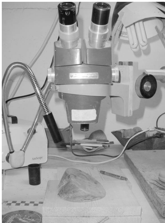
FIGURE 7. A focusing block set up in the field of view of the microscope. A fossil in Carbowax™ can be placed on it and worked from many different angles by spinning the block and the specimen, either together or independently.
