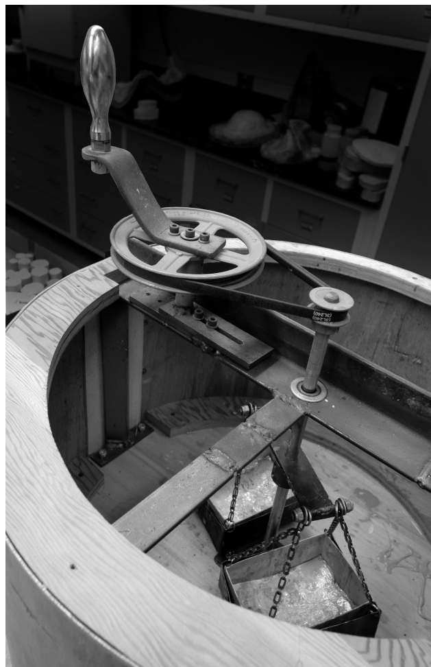
FIGURE 2: Centrifuge drive train assembly. The large drive pulley turns on a slotted belt tensioning mount.
