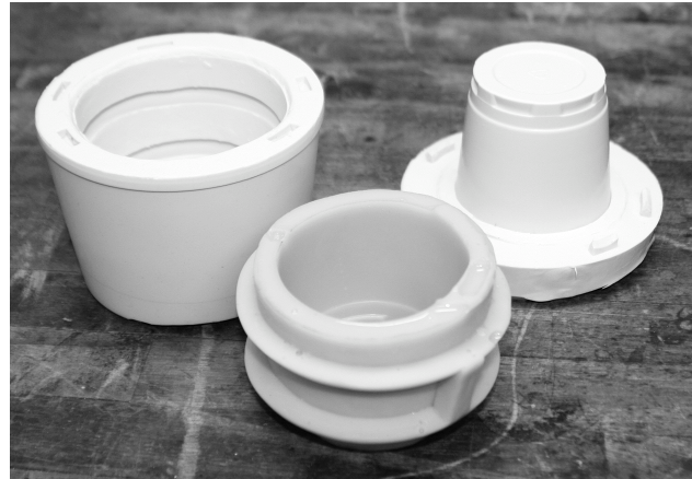
Figure 1: The polyurethane plug (foreground) is cup-shaped with walls about 1 centimeter thick. Two ridges and a vertical “key” position and secure the plug in the mold. I initially sculpted the form out of clay and then produced a silicone mold (two pieces in the background) from which we could produce numerous polyurethane plugs.
