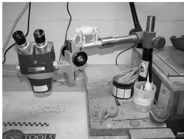
FIGURE 1. The essential tool for micropreparation; the binocular microscope on a boom. Other tools seen in immediate work area include three pieces of wood placed in the field of vision to elevate the working surface if needed, a dental pick, a poof, metal tin with scraps of paper, plastic tub with glue dispensers, hand exercise ball and rubber bands, sharpening stone, a paintbrush and a diamond nail file. The boom swings to the right in this photo allowing the microscope to be placed over the glass-covered sandblasting work chamber seen on the edge of the photo.
