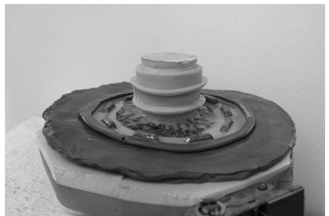
Figure 3: Because the plug is collapsible once the plaster support is removed, it is easily pulled out of the surrounding mold piece.
